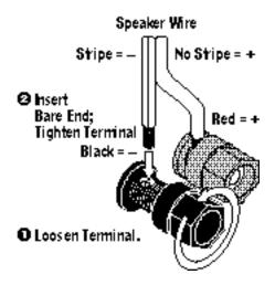
To ensure proper polarity, connect each + terminal on the back of the amplifier, receiver, or television to the respective + (red) terminal on each speaker, as shown in Figure 4. Similarly, connect the - (black) terminals in the same way. Also, see the owner's manuals that were included with your amplifier, receiver, or television to confirm connection procedures.
